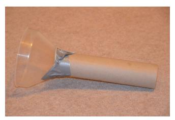
Attach the funnel to the cardboard tube using gaffer tape.
